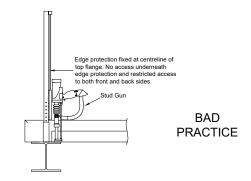
When selecting an edge protection system for use on floor levels where metal decking and stud welding operations will take place, the following placement considerations should be taken into account.
